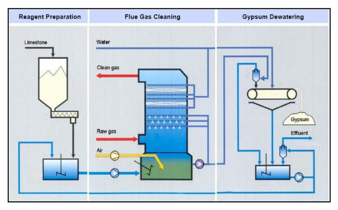
See Figure 2 for the process flow diagram for a typical FGD system operation.
